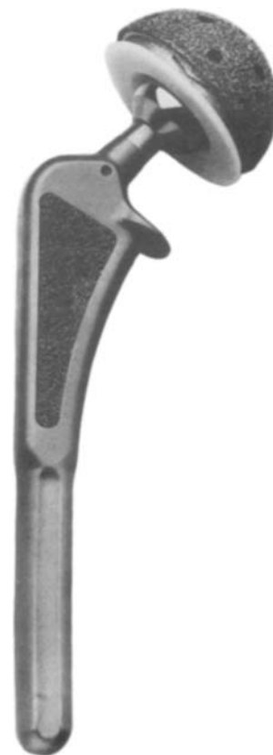
Figure 9 A total hip prosthesis system with titanium wire mesh sintered on to the surface of the stem and the acetabular cup for fixation by ingrowth of bone. (Courtesy of Zimmer Limited, Swindon, UK).
